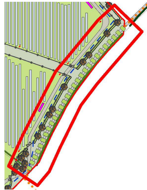
Green Lane 1 - 1:2500 @ A3 Minimum offset to panels: 13m Maximum offset to panels: 36m
