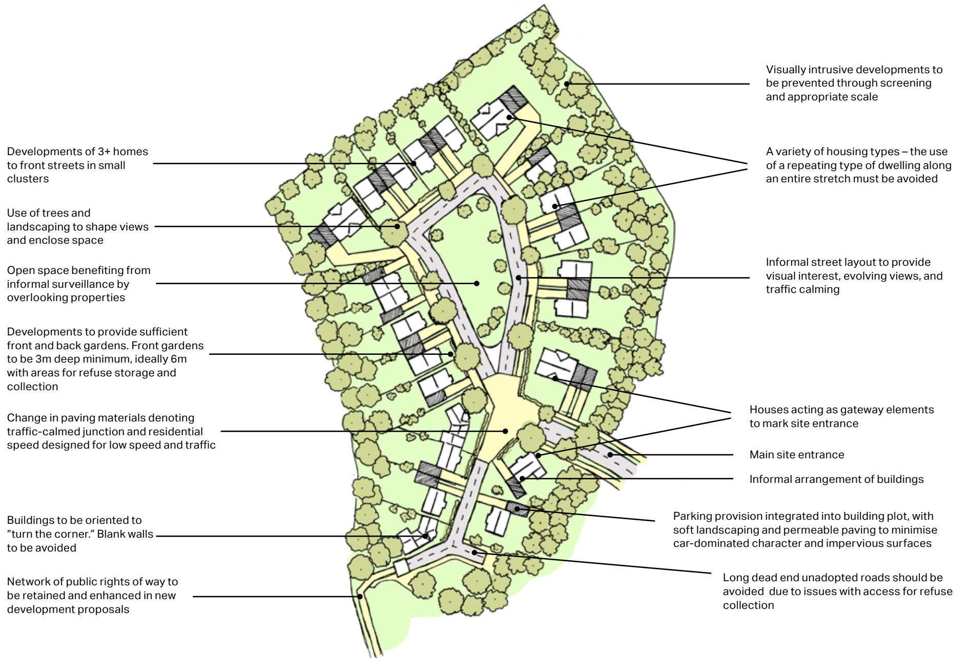
Figure 46: Illustrative plan for a small development highlighting many of the elements of the Bottesford code where they relate to the pattern and layout of buildings.
