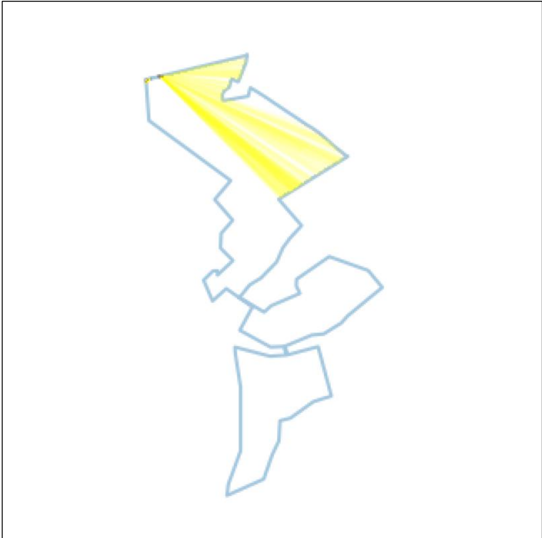
Figure 22 Reflective footprint for road receptor 24
